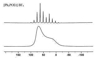
**Figure 2.**  $^{31}P$  CP/MAS spectra of polycrystalline [Ph<sub>3</sub>POEt]BF<sub>4</sub> (1) at 2 kHz (top) and 0 kHz (bottom) spinning speeds.
