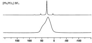
**Figure 1.** <sup>31</sup>P CP/MAS spectra of polycrystalline [Ph<sub>2</sub>PEt<sub>2</sub>]BF<sub>4</sub> (**14**) at 4 kHz (top) and 0 kHz (bottom) spinning speeds.
